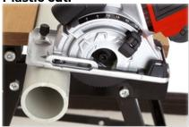
• For cutting plastic and aluminium always use HSS-saw blade (F)
