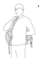
Put on the exoskeleton like a rucksack. When doing so, put on the shoulder straps without tightening the shoulder belts.
