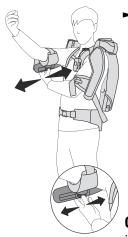
Checking the armrest position: With horizontal arms and elbows bent facing upwards, a distance of approx. four finger-widths should remain between the elbow and the armrest. The rubber straps of the armrests must not cut into the bends of the elbows here.
