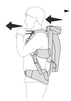
Pull the exoskeleton towards your back with the **position adjustment straps**.
