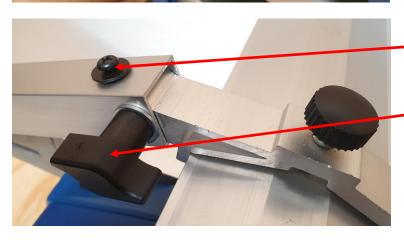
Slide the bridge guard into the end of the bridge guard arm and secure using the screw and washer.
