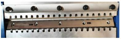
Once the new knife is in place, refit the locking bar.
