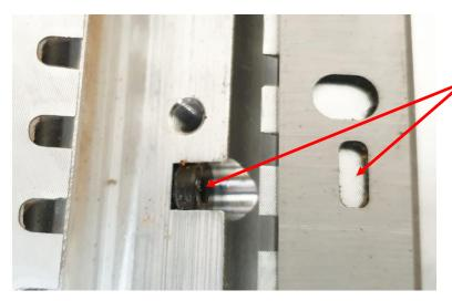
Place the new knife into the cutter block.
