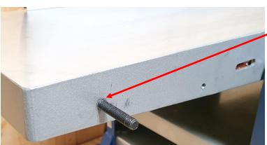
Fit the bridge guard arm pivot bolt
